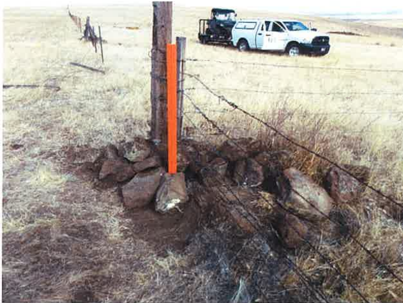
B . The established section corner with an orange carsonite post.
