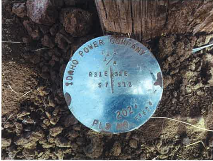
A . Set 30 X 2 1/2 in. aluminum post at the corner point alongside fence corner. As previously noted, the cap is stamped incorrectly.
