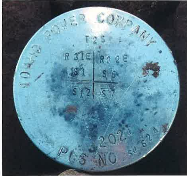
A . Set 30 X 2 1/2 in. aluminum post at the corner point alongside fence corner.
