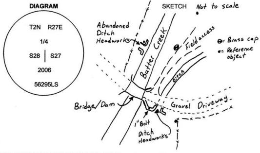
MONUMENT (S) AND ACCESSORIES SET (Procedures and Description) I set a 1 1/2" x 30" galvanized iron pipe with a 2 1/4" brass cap stamped as shown in the diagram above at the average intersection of fences North, West and South.
